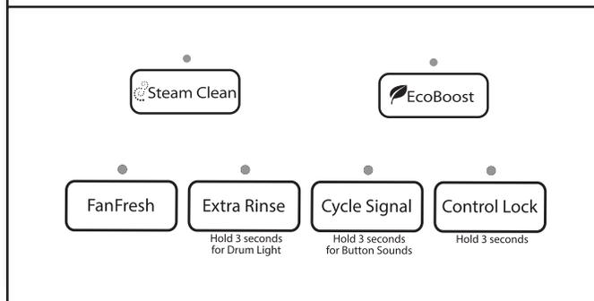
To add an option to the cycle, touch its name – Steam Clean, EcoBoost™, FanFresh®, Extra Rinse, Cycle Signal, or Control Lock. To remove an option from the selected cycle, touch the option again.
