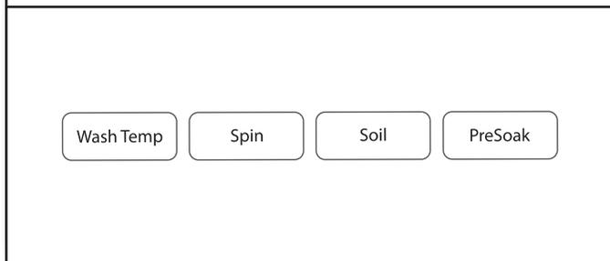
The display will show the default settings for the selected cycle. To adjust a setting, touch its name – Wash Temp, Spin, Soil, or PreSoak. Adjusting settings will change the Estimated Time Remaining. Tightly packing the load, unbalanced loads, or excessive suds may also cause the washer to increase the cycle time.
