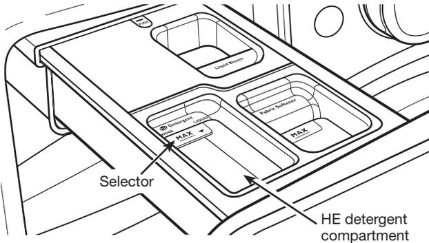
Pour a measured amount of HE detergent into detergent compartment. For powdered detergent, lift the selector to the high position. For liquid detergent, push down the selector to the low position.
