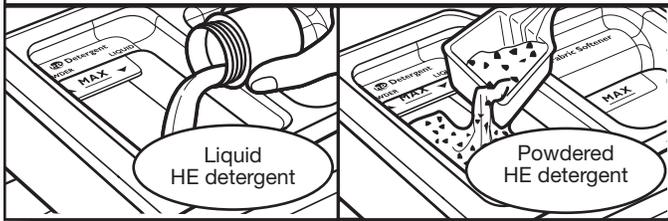
Adjust the selector, based on type of HE detergent used (either liquid or powdered). See “Using the Dispenser Drawer” instructions on how to use the dispenser.
