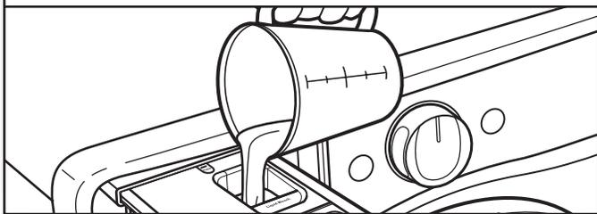
Add liquid chlorine bleach to the bleach compartment. Do not overfill, dilute, or use more than 2/3 cup (165 mL). Do not use color-safe bleach or Oxi in the same cycle with liquid chlorine bleach.
